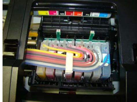
Arrange all the dampers and tubes; Gently press all the color dampers so they can sit firmly and connecting to each print head. Sometimes, you may need to push them a little bit harder so they can have much better connection to the print heads.
