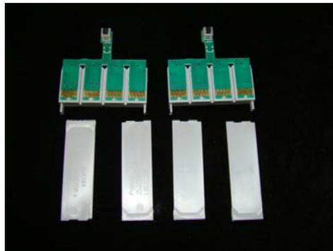
3. Install the chipset and chipset holders. If the Red LEDs are solid, then push the "Ink" button on the panel, and push two switches on the chipsets, then push "ink" button again on the printer panel.
