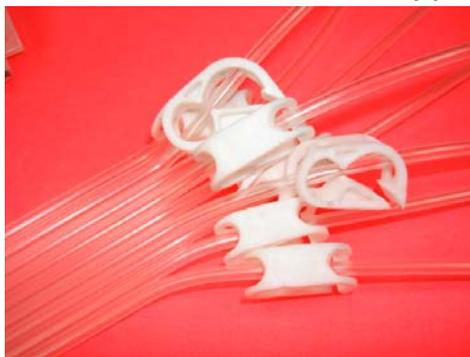
Install the sturdy ink tube (which will draw the inks from bottom of the bottle all way to the ink tube and damper). Then attach each ink tube to the bottle cap – make sure you match the color on both ink bottle and the damper/cartridge part. DO NOT mismatch the colors.
